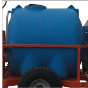
3,000 It Storage tank
