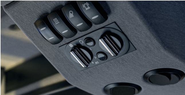
Instrumentation and air condition All switches are within easy reach on the overhead console. The optional air-con offers great comfort for the driver and passenger.
