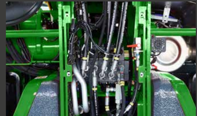
6 Best possible access to the control block.
