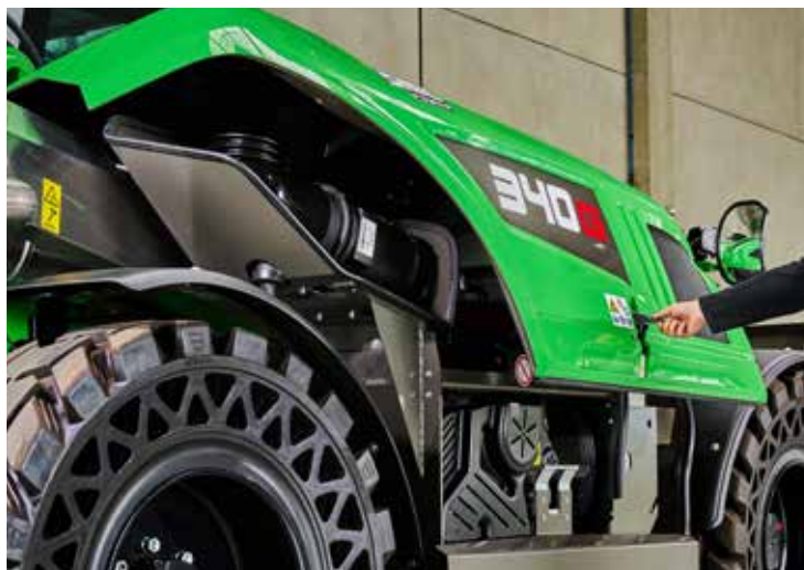
Spacious access to the engine compartment with just one handle. The side plate of the engine nacelle can also be removed.
