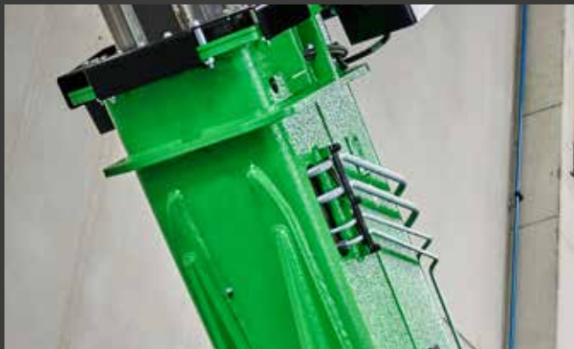
4 The pipes leading inwards are optimally protected from damage by the boom and ensure a safe supply of hydraulic oil.
